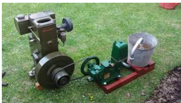
A Lister D with a Lister Domestic water pump
